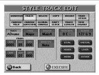
ERASE allows you to selectively delete data either within a specified range of measures, beats or clocks or from the entire track(s). When DATA TYPE is set to "ALL", ERASE substitutes the required number of rests for the data you delete, so that you end up with the equivalent number of blank measures. If you also want to eliminate the measures themselves, use DELETE (see below).
